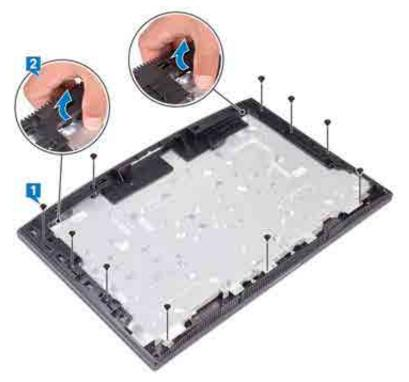
**3** Lift and slide the middle frame off the display-assembly base.
