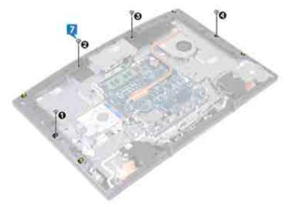
8 Remove the four jig screws from the display panel.
