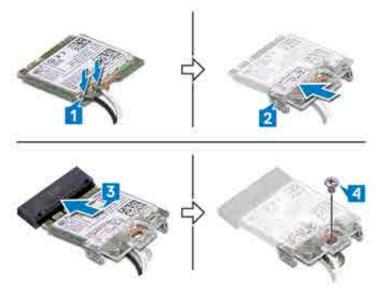
6 Place the wireless-card shield on top of the wireless card.
