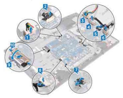
**11** Remove the six screws (M3x5) that secure the system board to the displayassembly base.
