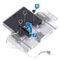
8 Pull the clip on the retractable-camera assembly, and rotate the camera and camera bracket along with the camera cable, off the retractable-camera assembly.
