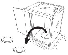
**1** Remove the anti-draft ring, the pan, and the pan supporter from the weighing chamber
