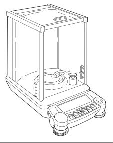
Load and unload a weight close to the capacity 6 times
