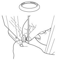
**2** Unscrew and remove the inside knob on the glass door.
