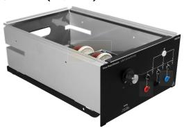
The Three-Phase Rheostat module consists of three rheostats mounted on a common shaft directly controlled by a single knob on the module faceplate. The rheostats are electrically interconnected in a four-wire wye configuration and each leg is protected from over-current conditions by a thermal-magnetic circuit breaker.
