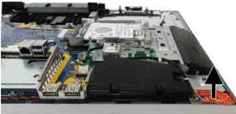
To replace the audio board, reverse the removal procedures.
