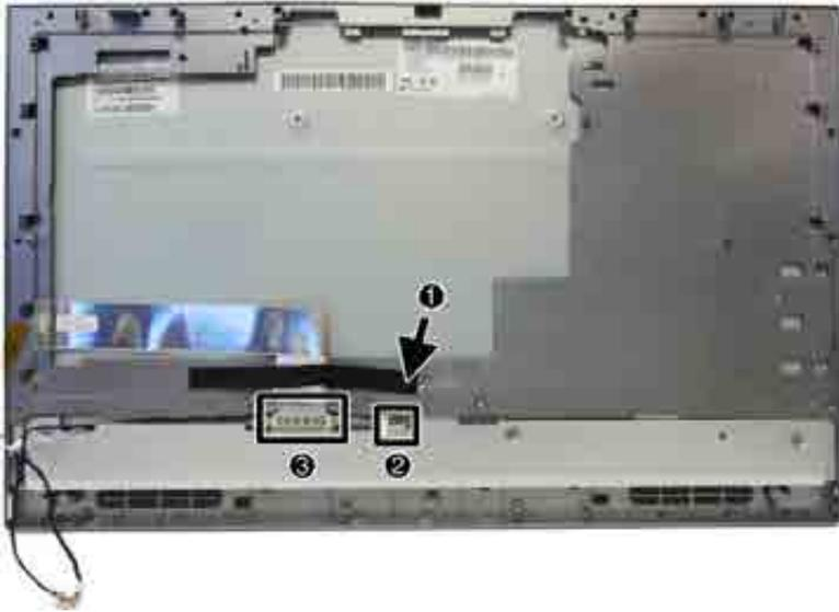
18. Separate the middle frame from the display by rotating the top of the display away from the frame (1), and then pulling the frame away from the display (2).
