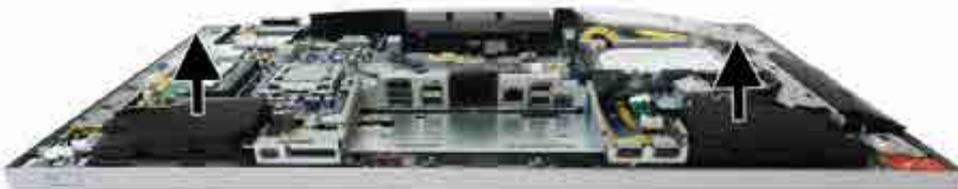
To install the speakers, reverse the removal procedures.
